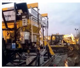
Keltbray Rail has developed a new and unique mobile batching plant for concrete foundations works on railway projects.
