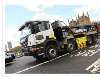
Keltbray was also first to equip its vehicles with the Dawes PeoplePanel™. These panels are specifically made of a specialist grade of tough shatterproof plastic that are fitted over existing under-run bars to reduce the risk of entanglement of clothing or bicycle parts.
